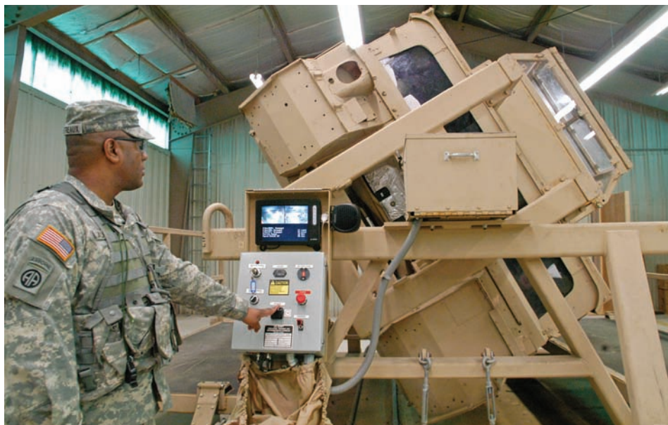
Top: Staff Sgt. Winston Gautreaux demonstrates how the High-Mobility Multipurpose Wheeled Vehicle Egress Assistance Trainer simulates a Humvee rollover. The vehicle, which seats four, can spin 180 degrees in nine seconds.
